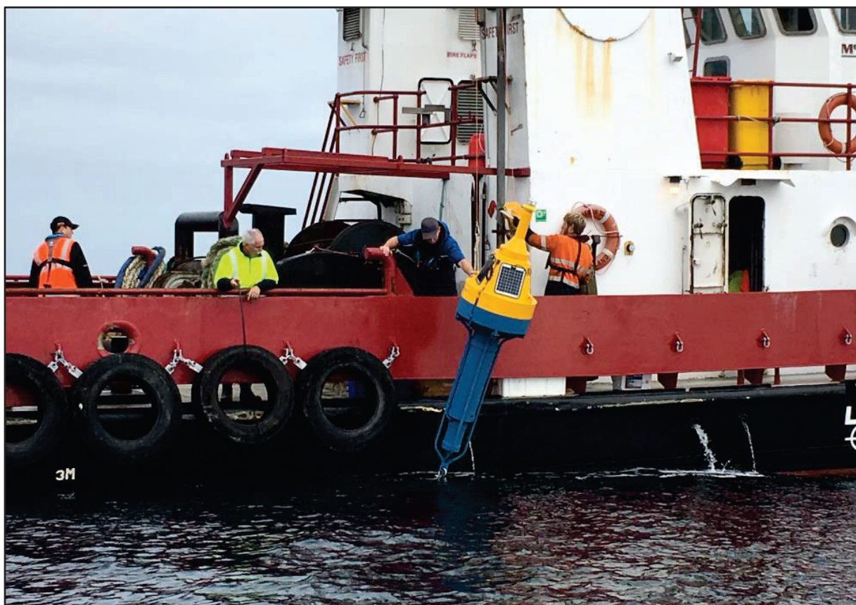
Figure 4.3: Deployment of ADCP and WQM Devices
