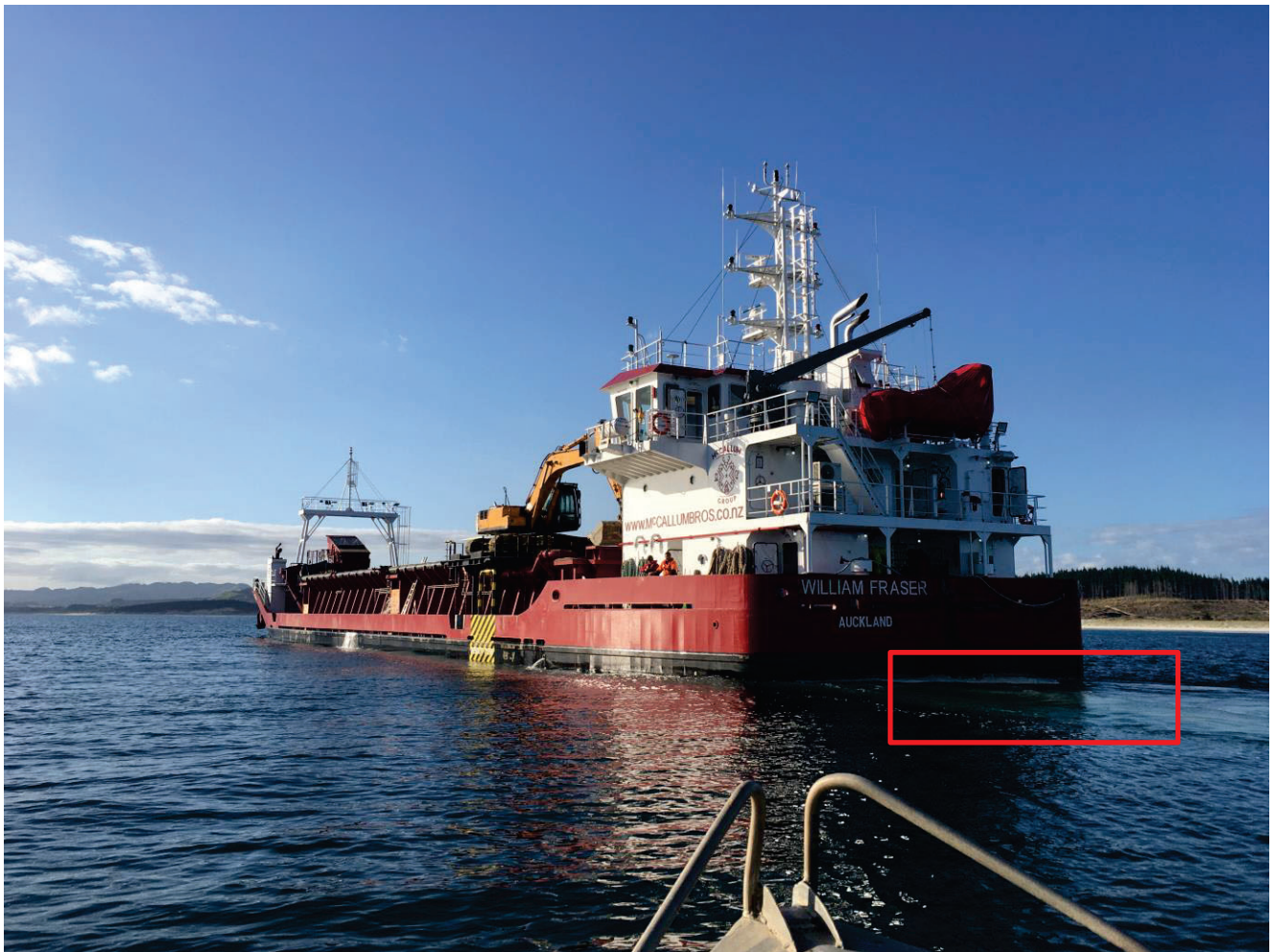
Figure 5.3: Location of Survey Vessel at Start of Sand Extraction Plume Sampling. The sampling vessel was positioned approximately 3 m from the vessel stern
