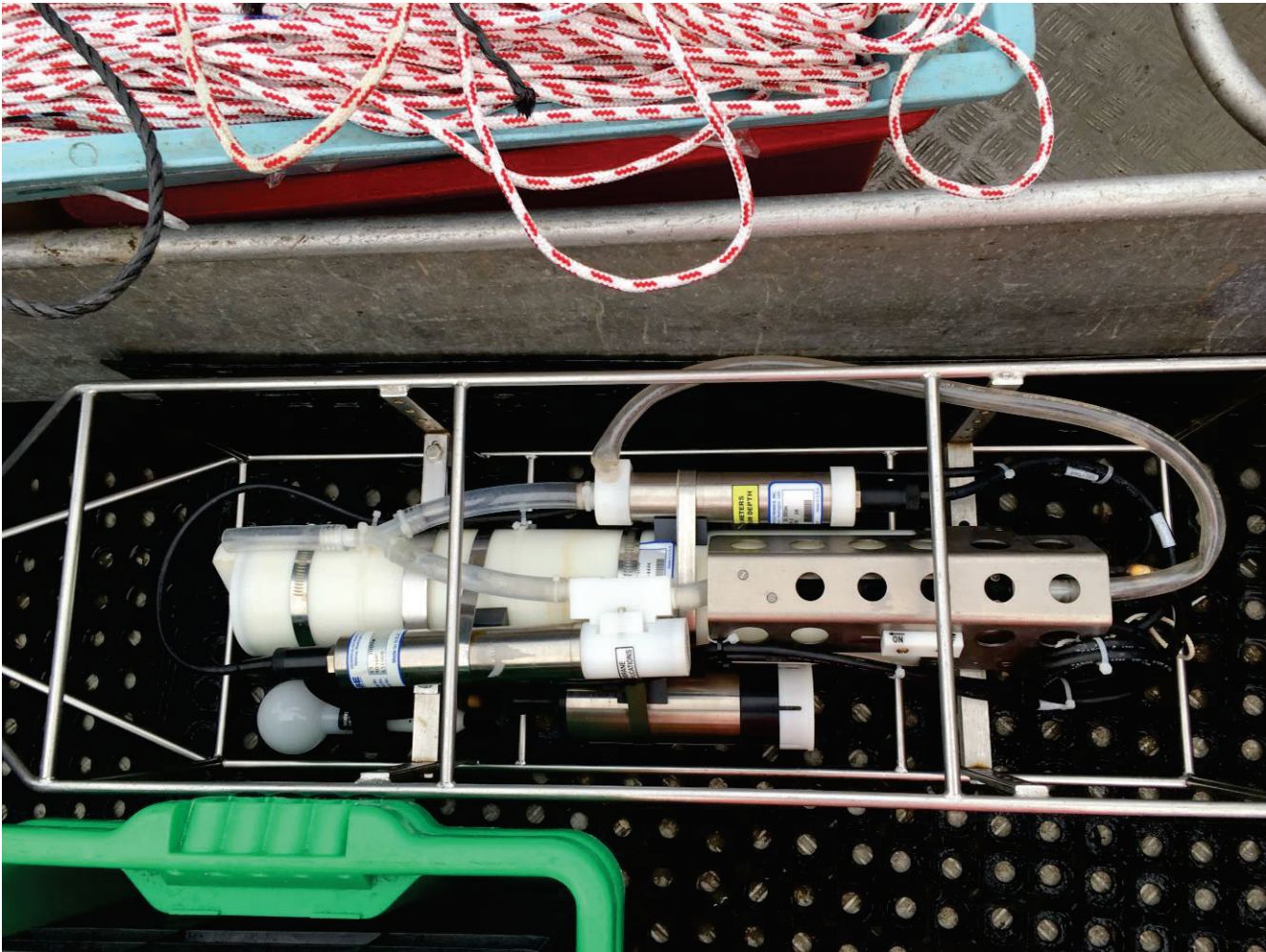
Figure 4.5: CTD Instrument with Integrated Fluorometer
